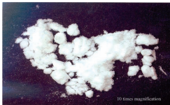
Figure 1. Photograph of the precipitate obtained using synthetic water containing struvite components in stoichiometry proportion at pH 9 (sample P-1).
